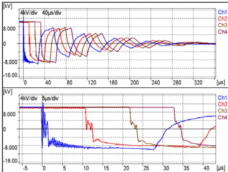
Fig. 6 : Measurements with different divider configurations
