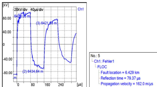
**Fig. 13 :** Analysis of the reflection measurement
