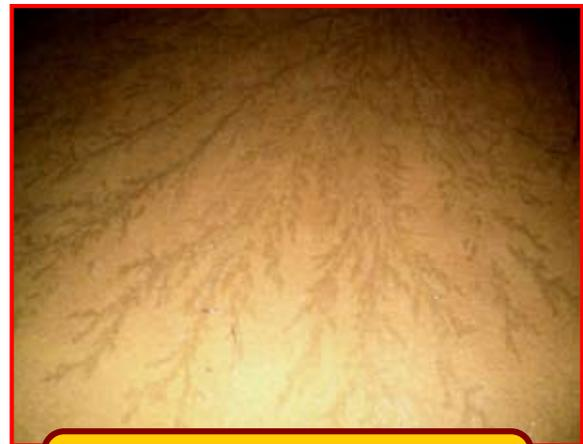
Tree formation crepage path due to dust particle on Paper Insulation.
