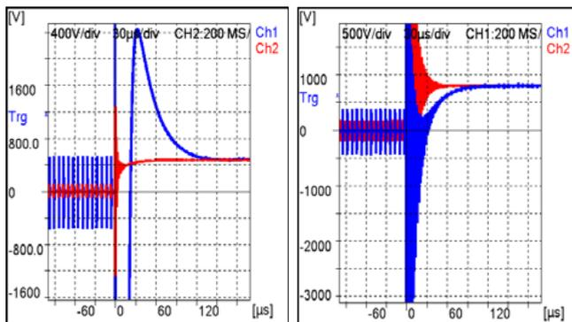
Fig. 9 : Step response of divider A (left) and divider B (right), undamped (Ch1) and damped (Ch2)
