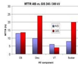
Failure rates and Mean Time To repair (MTTR)
