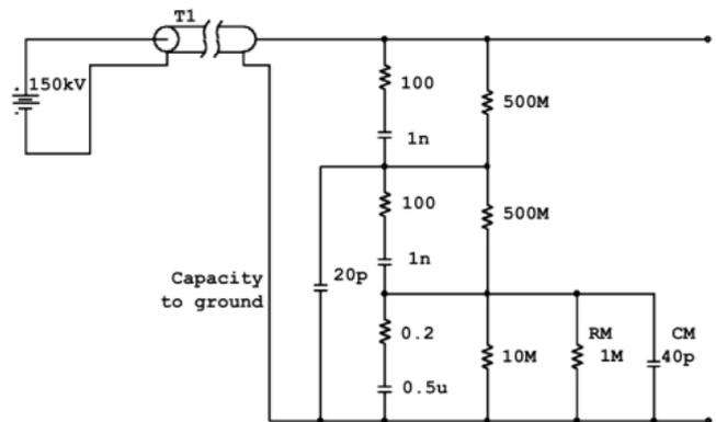
Fig. 2 : Simulated cable
