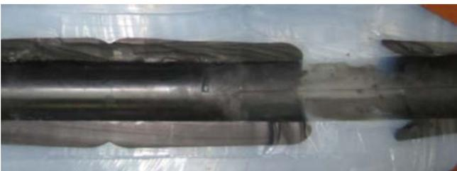
**Fig. 14 :** Faulty cable sleeve
