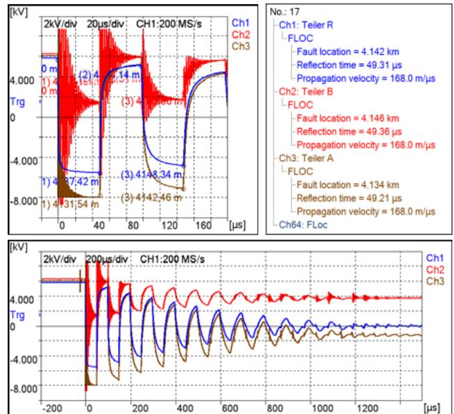
Fig. 10 : Sample measurements on divider A, divider B and divider R
