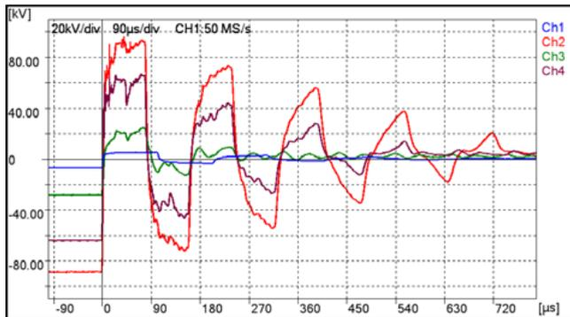
**Fig. 12 :** Three breakdowns at different voltages (Ch1 is the reference measurements)
