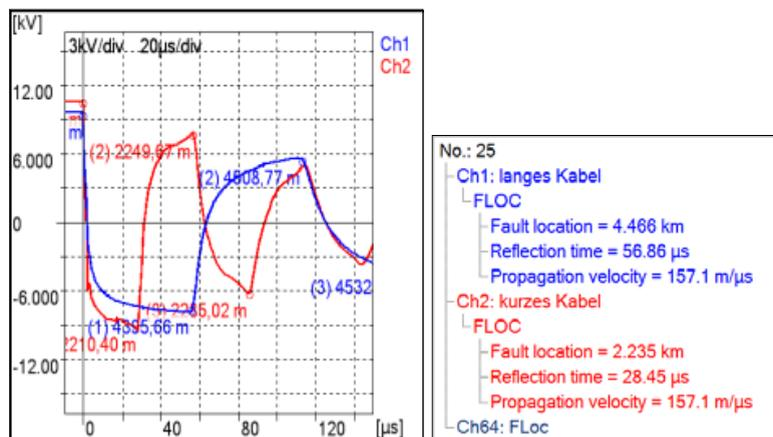
Fig. 7 : Measurements on single- and double-length cables
