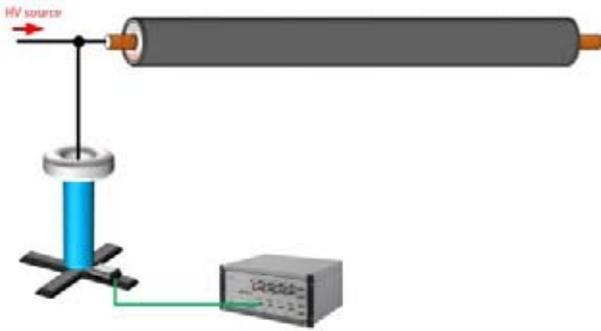
Fig. 1 : Basic measurement configuration for online fault location
