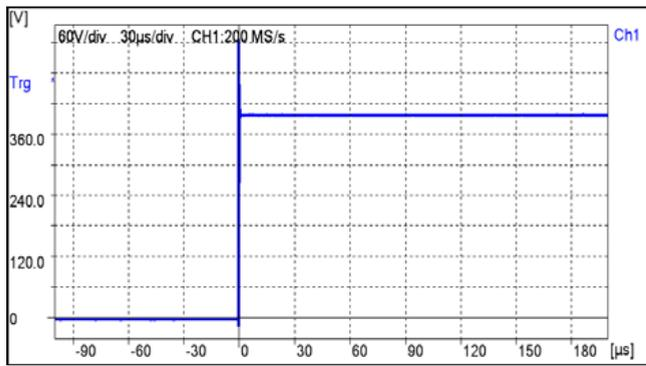
Fig. 8 : Step response of divider R,  $t_s = 180$  ns
